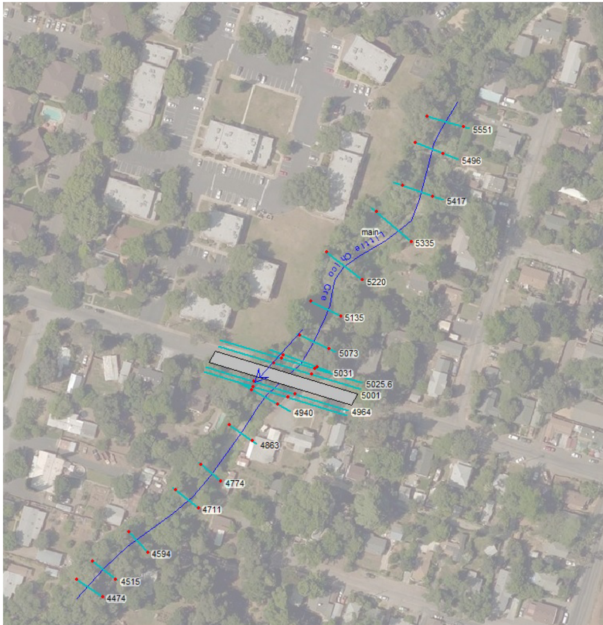
Figure 5. Plan View of HEC-RAS cross sections
